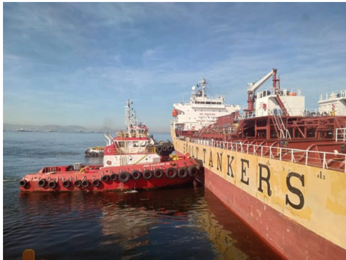
Figure 2: Tanker Stolt Kiri , 146 metres length, assisted by two powerful ASD tugs José Guilherme VIII , 32 metres length, 62 tons bollard pull and Diamante , 32 metres length, 62 tons bollard pull
