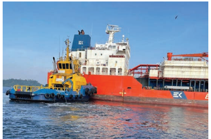
Figure 1: LPG tanker BWEK Antere , 120 metres length, assisted by ASD tug SAAM Antares , 32 metres length, 80 tons bollard pull. Note the side wash of the tug
